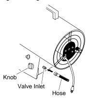
Figure 7 - Hose and Inlet Connector
